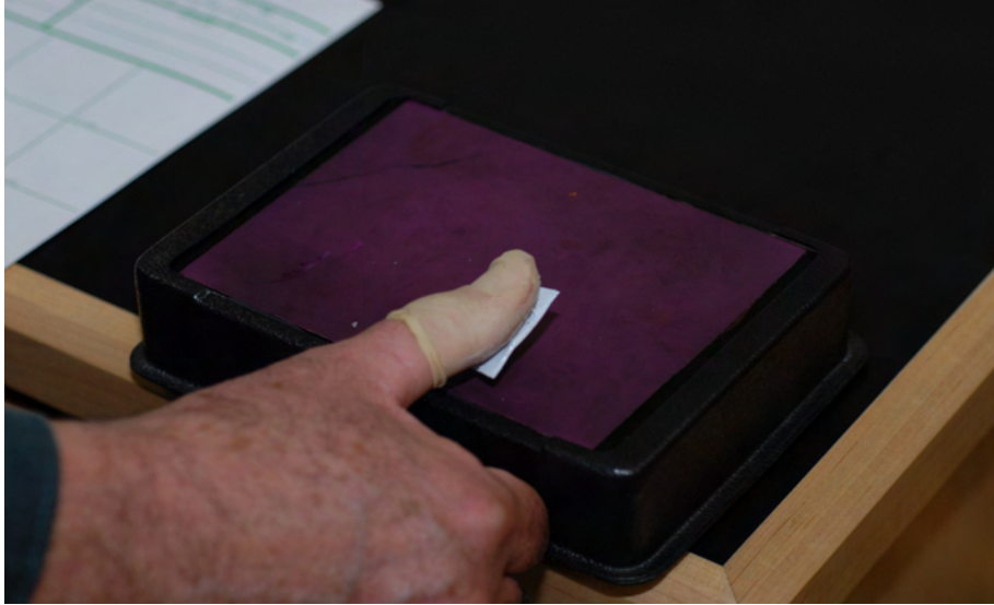
Mikrosil® cast affixed to a latex glove and applied to an inkless fingerprinting system.
